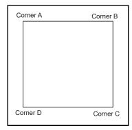
It is important to first insert graphic into each alternate corner, then to the sides of the frame. If this is not done, graphic will not fit into the frame correctly.
