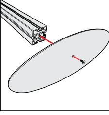
Base Plate & Extrusion Connection
