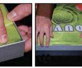
Step 3 Once all corners are inserted. press one silicon edge into channel from corners and work toward the center. Make sure welt is fully inserted into channel. Continue until all sides are done. Smooth out edges of graphic.
