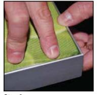
Step 2 Repeat Step 1 for opposite corner C, then insert corner B, followed by corner D, to complete the installation of the corners.
