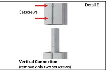
When vertical extrusions are packed in portable cases rather than crates or tubs, they must broken down into smaller sections which then require assembly.
