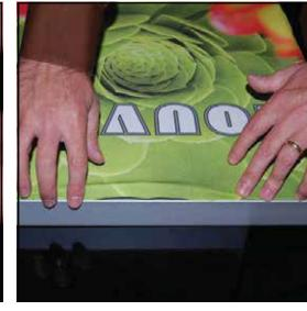
Once all corners are inserted, press one silicon edge into channel from corners and work toward the center.
